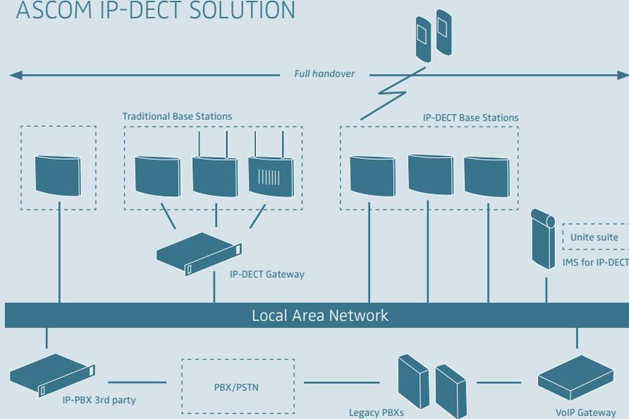
Older handsets such as DT288, DT290, DT368, DT570, TH688 and 9d23 as well as Ascom's latest handsets, DT292, OfficeT, DT590, OfficeM and 9d24, are compatible with our IP-DECT solution. This backward compatibility with older handsets means that any DCT1800-GAP, MD Evolution, BusinessPhone or MD110 system, running DECT GAP and/or CAP can be replaced by IP-DECT.
